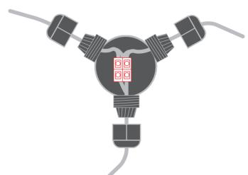
**3.** Tighten the plastic nuts with the flat wrench.
