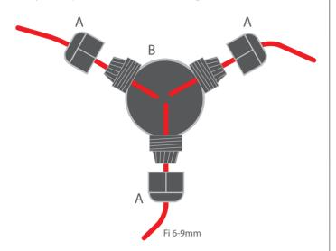
**2.** Connect the cables using e.g. a connection block and place the connection inside the body.
