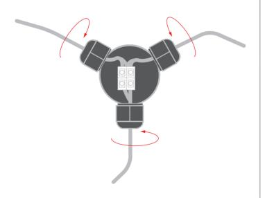
4. Put the lid (C) on the body and twist it shut
